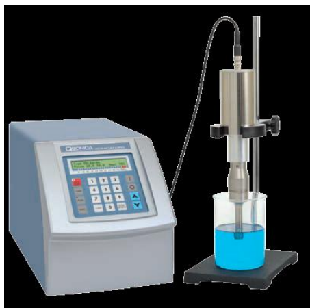
Fig. 2. A sonic horn, or sonotrode, immersed in a liquid for sonication. Courtesy of Qsonica LLC, Newtown, CT, USA.
